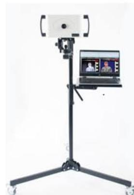
The WG520 Fever, Coronavirus, Flu, Ebola Screening System is a portable rapid deployable thermal imaging fever screening system that is used as a first level mass screening test for accurately identifying individuals that have an above normal body temperature and have a systemic fever and may be suffering from Coronavirus, Ebola, Common Influenza, Norovirus SARS and other flu variants such as Avian Flu, Bird and Swine flu etc.
